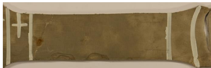
5.6 specimen – FE (top) and experimental (bottom) failure mode – the experimental specimen failure near the support due to the excessive corrosion in that region
