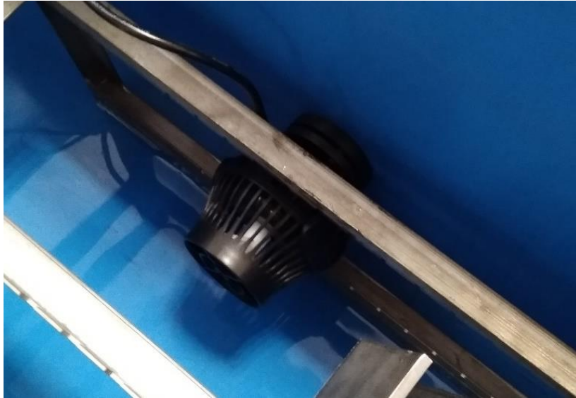
Figure 4.5. A circulation pump was used during corrosion testing.
