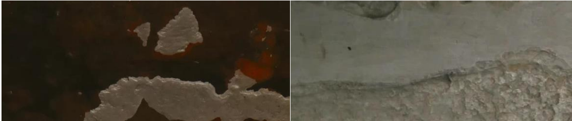
Figure 4.15. The example of a specimen before (left) and after (right) cleaning.
