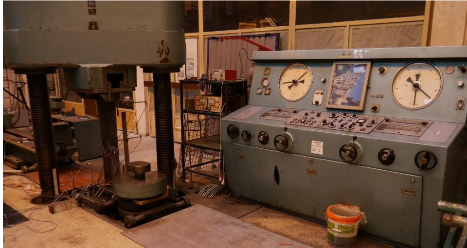
Figure 6.13. Testing machine with the mounted specimen (left).
