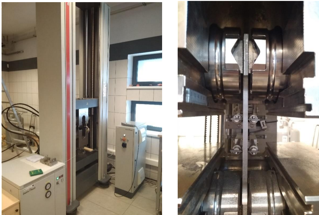
Figure 6.27. Testing machine (left) and mounted specimen with installed extensometer (right).
