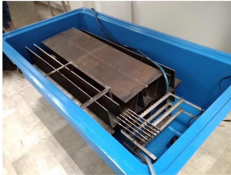
Figure 4.4. Corrosion tank with placed specimens.
