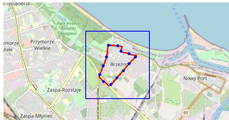
Figure 3. The software map area. The blue rectangle is the extent of the loaded DSM. The red line is an inspected route. The blue dots are sampling points where DOP values were calculated.
