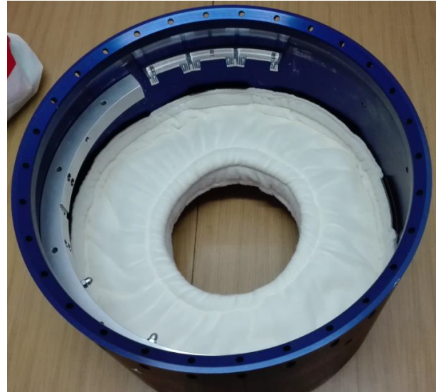
Fig. 9. Insulation placed on thermal experiment.
