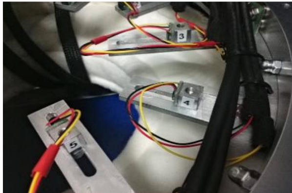
Fig. 5. Cantilever beams (5 out of 8) inside REXUS 25 rocket [11].
