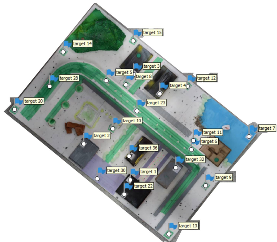
Figure 3. Positions of F-points (marked with blue flags with the target and number inscription).
