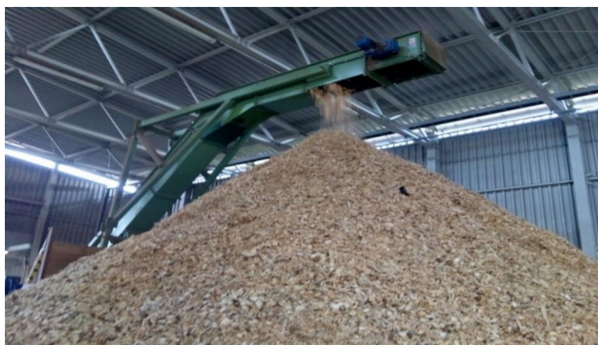
Figure 4. Chipper for biomass homogenization in Lębork (photo: B. Igliński).
