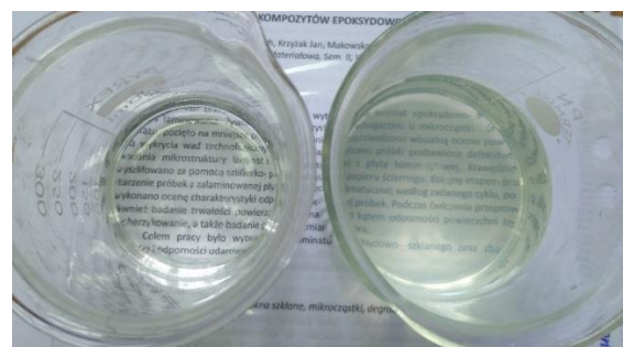
Fig. 2. Comparison optical transparency, a) neat diesel fuel b) nanofuel – \text{Al}_2\text{O}_3 50 ppm, turbidity ~30 NTU
