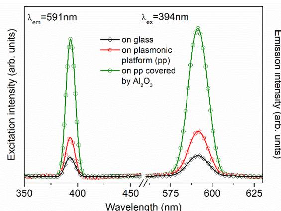
**Figure 5.** Excitation and emission spectra for TiO<sub>2</sub>:Eu thin film deposited on a Corning glass substrate and TiO<sub>2</sub>:Eu film deposited on plasmonic platform in a both configurations, without and with additional dielectric layer.
