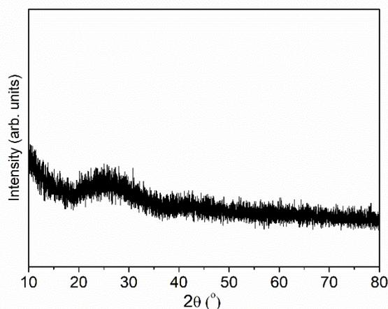
**Figure 2.** XRD pattern of TiO<sub>2</sub>:Eu thin film, deposited on Corning 1737 glass substrate.
