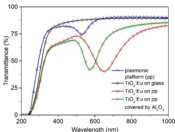
**Figure 4.** Transmittance spectra for TiO<sub>2</sub>:Eu thin film deposited on a Corning glass substrate and TiO<sub>2</sub>:Eu film deposited on plasmonic platform in a both configurations, without and with additional dielectric layer. Additionally spectrum for plasmonic platform is presented.
