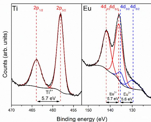
**Figure 3.** XPS spectra recorded for Ti2p and Eu4d core shell electrons of TiO<sub>2</sub>:Eu luminescent thin film.
