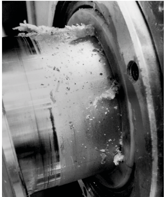
Fig. 6. Disassembly of bearing's cover: lubricating grooves clogged with wear particles. Test conditions: pressure=0.2 MPa, shaft revolution speed =10 rev/s, water flow=0 L/min.
