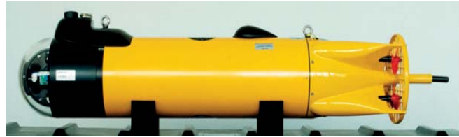
Fig. 1. Side view of the Gluptak vehicle. Length of the vehicle is 1.4 [m] and hull diameter is 0.25 [m]. Length of the stern, propulsion section is limited to 0.33 [m]
