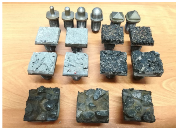
Figure 9. Different penetrators used in this study.
