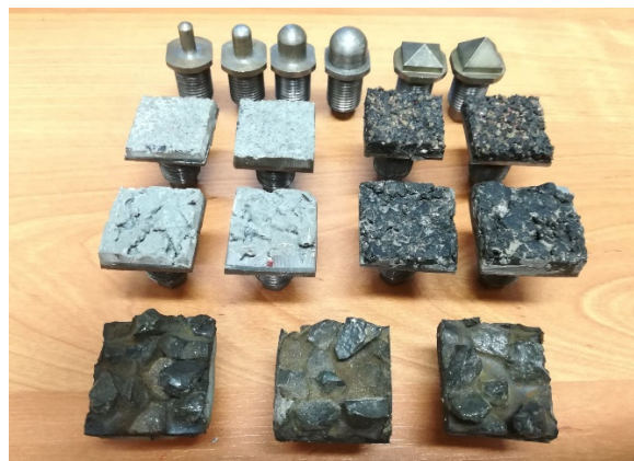
Figure 9. Different penetrators used in this study.
