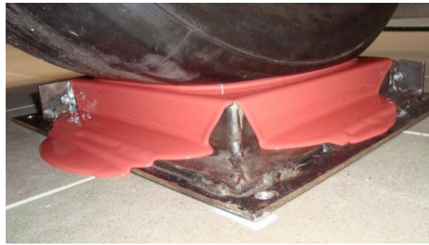
Figure 6. Making the contact deformations mold.
