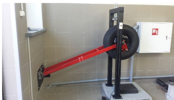
Figure 5. Facility to test dissipation of energy in tire by oscillation method.
