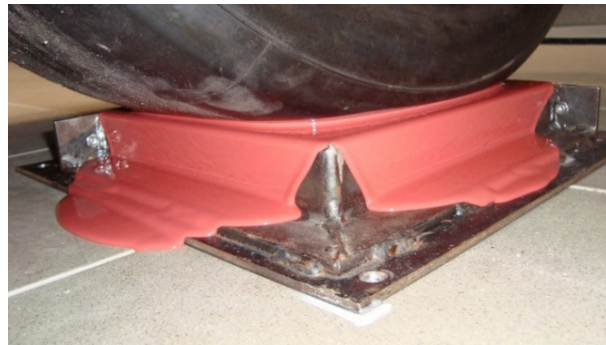
Figure 6. Making the contact deformations mold.
