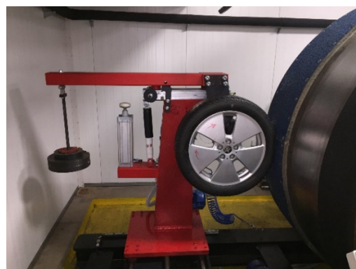
Figure 3. Roadwheel facility for tire rolling resistance measurements.
