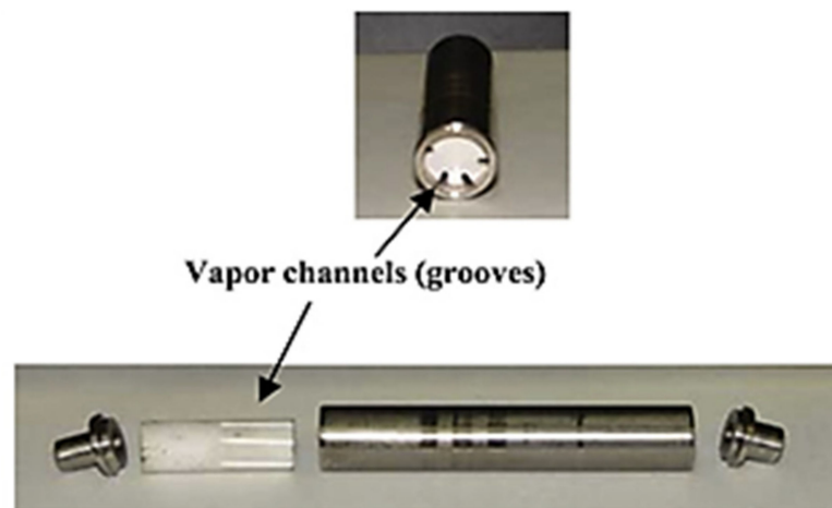
Figure 12. Ceramic wick with vapor channels (grooves) used in the LHP [45].
