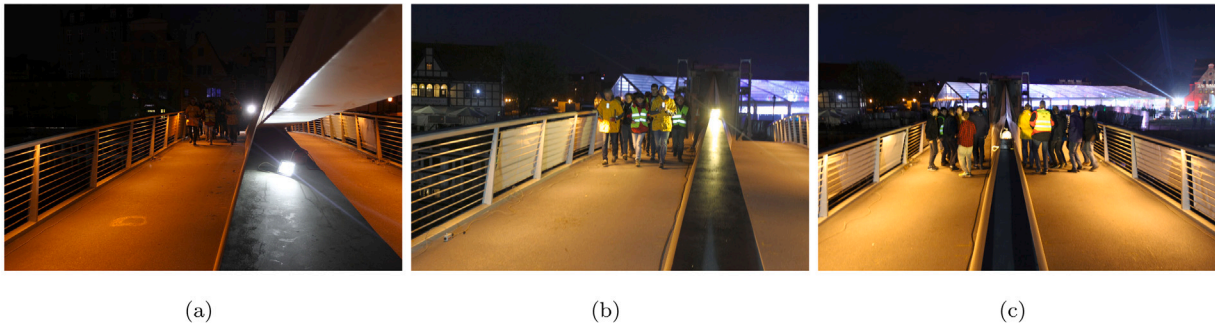
Fig. 22. Dynamic tests performed on the footbridge: (a) synchronous march, (b) synchronous and free running, as well as (c) squatting of groups of twenty pedestrians.
