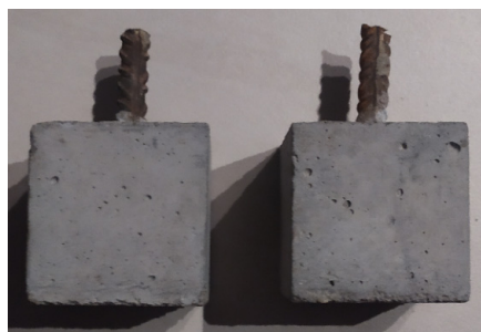
Figure 1. Reinforced concrete cubes for experimental procedure.
