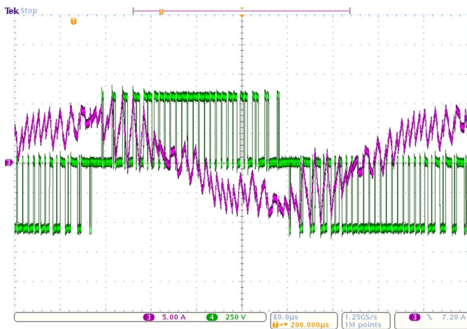
Fig. 6. Voltage and current waveforms of the stator of a 3.4 kW induction motor installed in the tested system with a silicon carbide inverter at voltage frequency of 1.5 kHz measured before the sinusoidal filter
