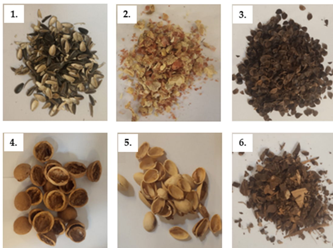
Figure 1. Raw materials: sunflower hulls (1), corncob (2), coconut shells (3), walnut husks (4), pistachio husks (5), buckwheat husks (6).
