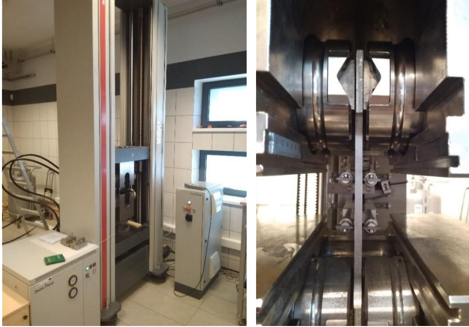
200 Figure 5. Testing machine (left) and mounted specimen with installed extensometer (right).
