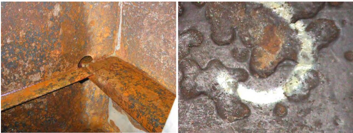
41 Figure 1. The comparison between general (left) and pitting corrosion (right) [6].
