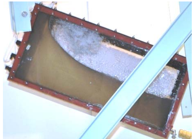
Figure 2. Exemplary shape of a free surface of liquid inside a partly filled model tank (own research) – it may be clearly seen that the free surface is far different than assumed within the quasi-static approach (ref. to Fig. 1)
