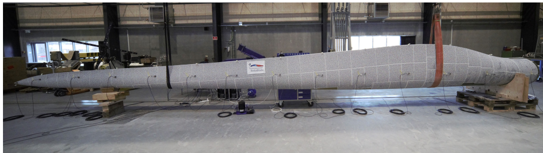
Figure 1: Wind turbine blade supported in a free-free boundary conditions on a test stand.
