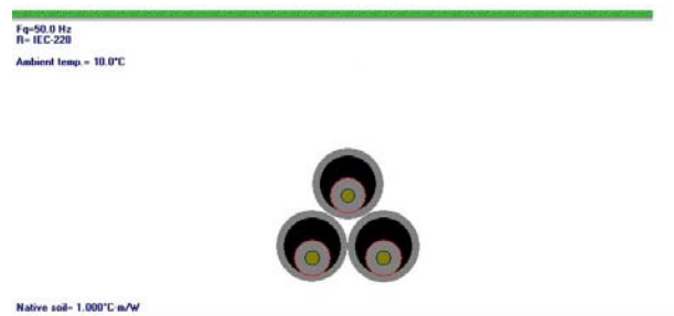
Fig.4. The arrangement of the analyzed power cable system; cables in pipe-type ducts: trefoil formation, thermal resistivity of the native soil 1.0 (K·m)/W, ambient temperature (soil) 10 °C
