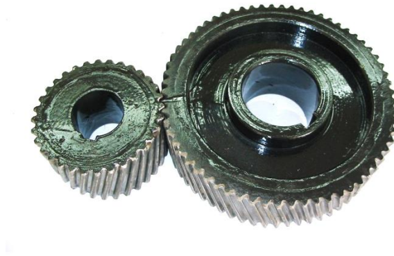
Fig.9. Photograph of the experimental non-circular gears (1-column image, colour online only)
