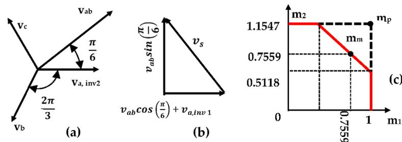
**Figure 3.** Operational boundary definition: (a) 3-phase phasor diagram; (b) components of the system's voltage magnitude,  $v_s$ ; (c) boundaries of the different and common frequency modes of operation.
