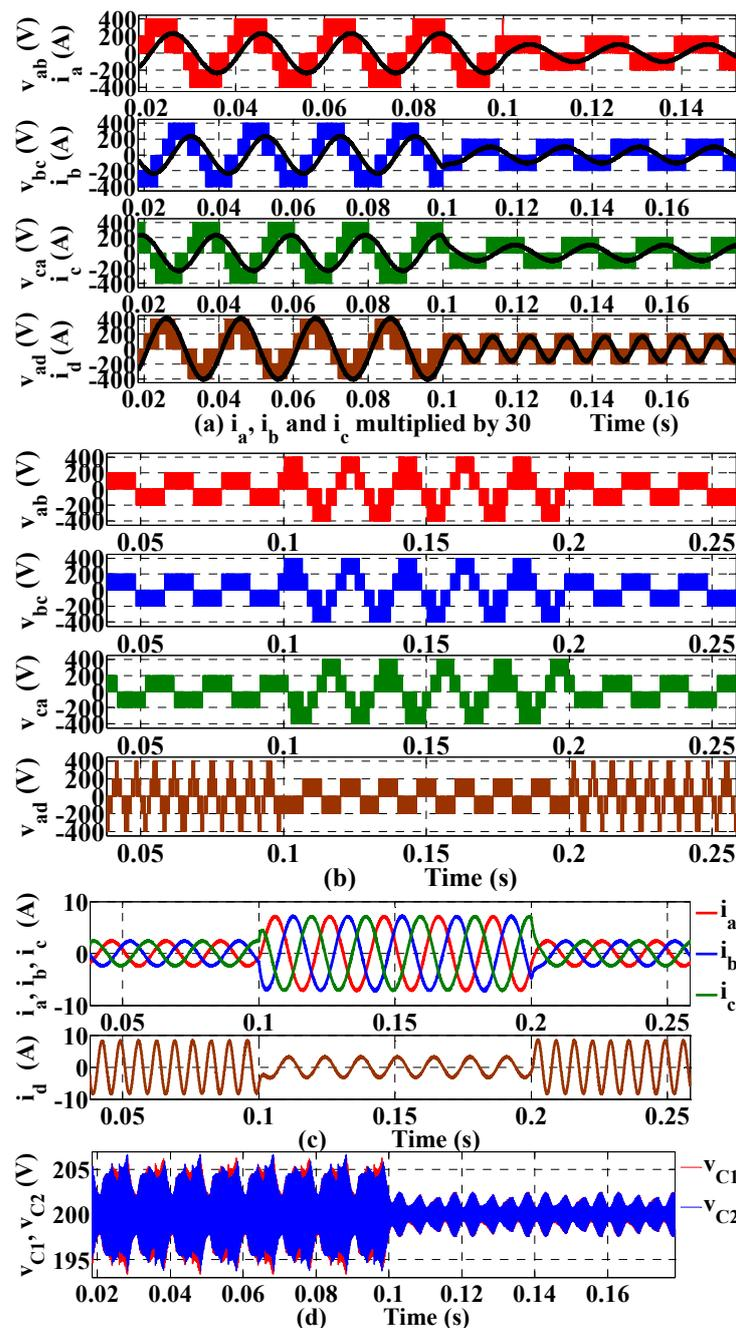
**Figure 7.** Simulated output voltage and current waveforms of the dual-phase inverter for common and different frequency operations. (a) Common 50 Hz and modulation indices of 1.1547 and 1 at frequencies of 50 and 100 Hz, with common modulation index of 0.7559; (b,c) different frequencies of 50 and 150 Hz, with modulation indices of 0.35 and 0.8 at different frequencies of 50 and 75 Hz, with modulation indices of 1.05 and 0.25; (d) capacitor banks' voltages in (a).
