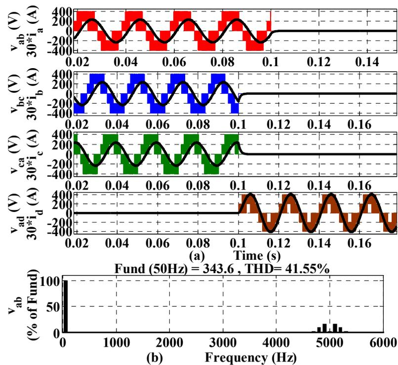
**Figure 8.** (a) Simulated voltage and current waveforms for either operation of the two inverters for common frequency of 50 Hz and modulation indices of 1.1547 and 1, (b) corresponding FFT profile of the line voltage waveform,  $v_{ab}$ , for this point of operation.
