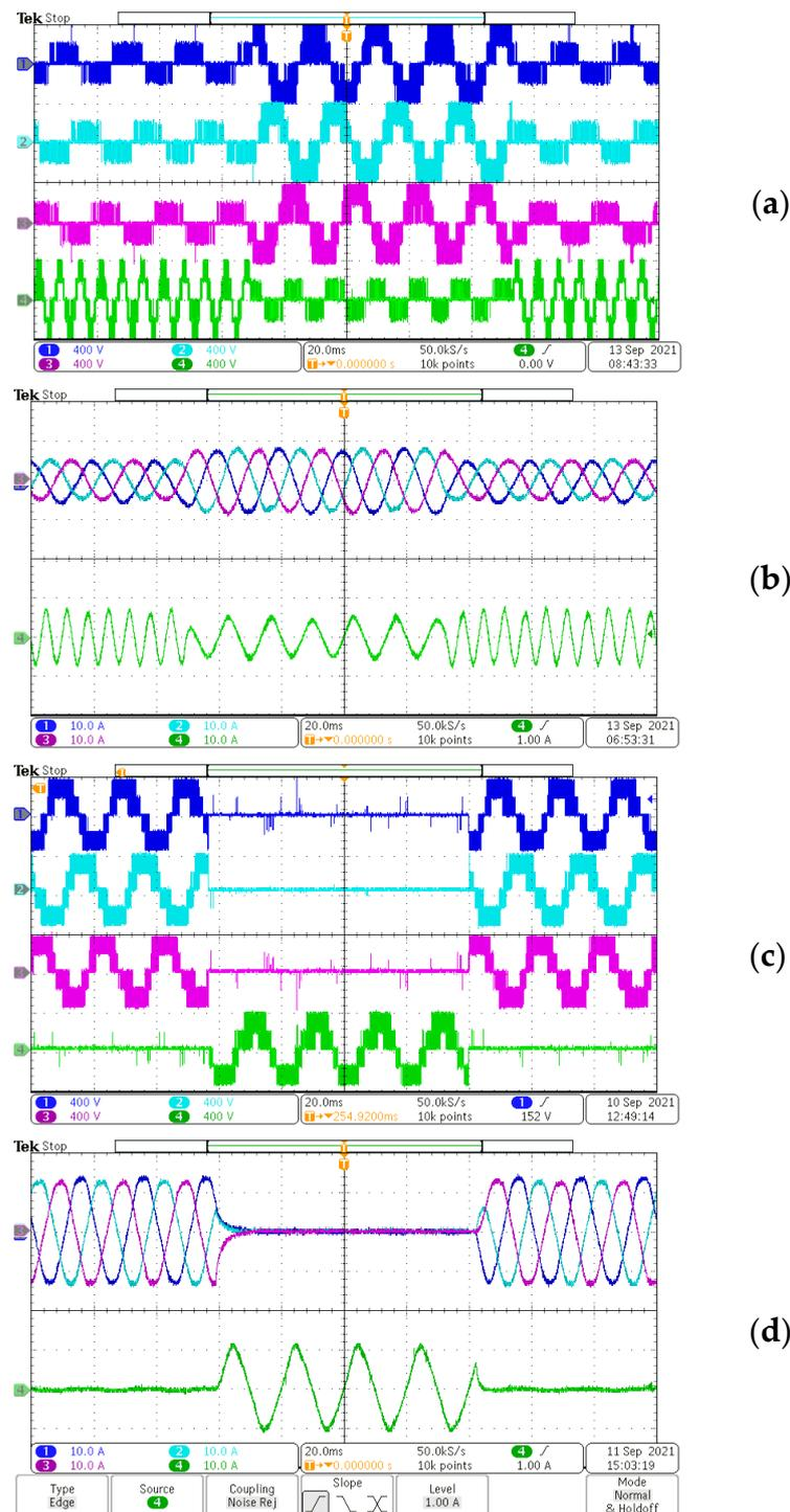
**Figure 10.** Experimental output voltage and current waveforms of the dual-phase inverter for different frequencies and modulation indices. (a,b) Output voltage and current waveforms for frequencies and modulation indices for inverters 1 and 2 of: 50 and 150 Hz, with modulation indices of 0.35 and 0.8 (50 Hz), and 50 and 75 Hz, with modulation indices of 1.05 and 0.25; (c,d) either operation of the two inverters at a common frequency of 50 Hz and modulation indices of 1.1547 and 1.
