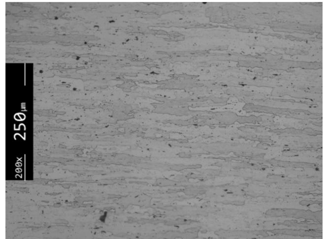
Fig. 1. Optical micrograph of the high-strength 7050-T6 aluminium alloy in the transverse direction [37].
