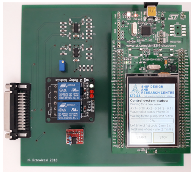
FIGURE 10. The wave maker embedded system, equipped with the STM32F4 microcontroller and graphical user interface [40].
