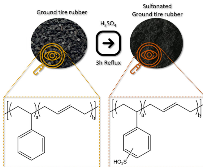
Fig. 6. Preparation of sulfonated GTR (adopted from Islam et al., 2018).
