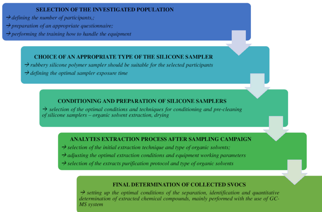
Fig. 3. Main stages of analytical procedures applied to determine SVOCs by rubbery silicone polymer personal passive samplers.
