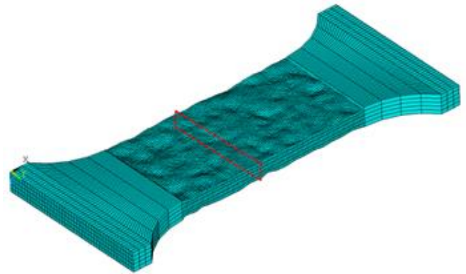
Figure 4. FE model of the specimen with randomly generated random fields of corrosion.
