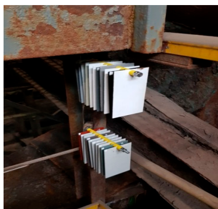
Figure 5. Mounted samples in the hall in a vibration-free place.
