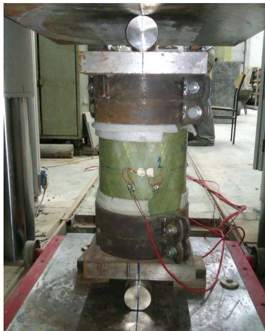
Fig. 9. Longitudinal compression test of the tube composite
