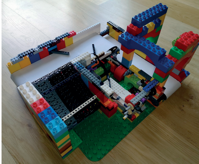
Fig. 39.1. Stand and conveyor belt for video recording. The camera was placed on the stands in the right side of the construction
