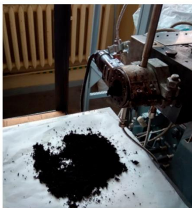
Figure 2. The appearance of GTR directly after auto-thermal reclaiming.
