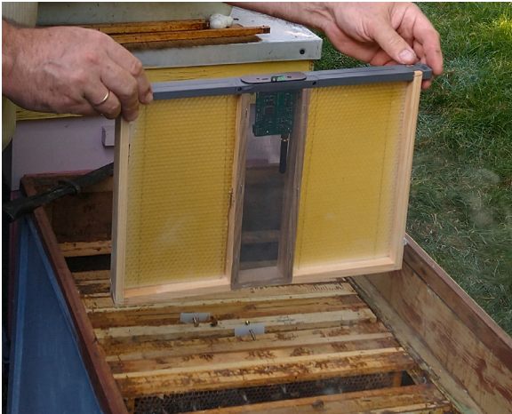
Fig. 2. Custom frame for collecting sound recordings placed in the center of monitored hive.
