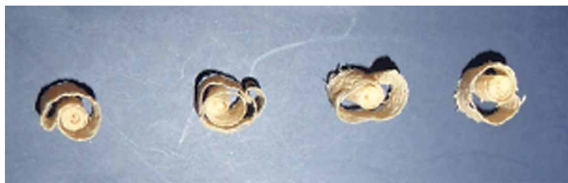
Figure 5 Exemplary collected chips from orthogonal cutting on sliding microtome in longitudinal direction to pine wood fibres; chips were created during cutting process with set uncut chip thickness h = 0.15 mm
