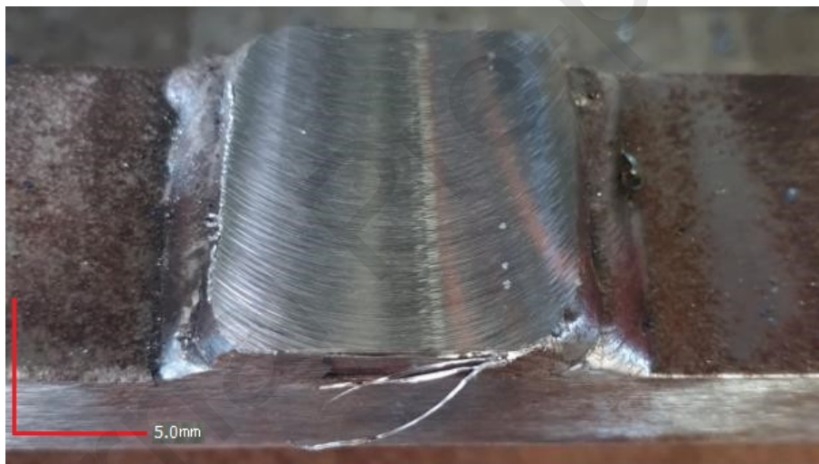
Figure 9. Cavity observed in triple weld specimen.
