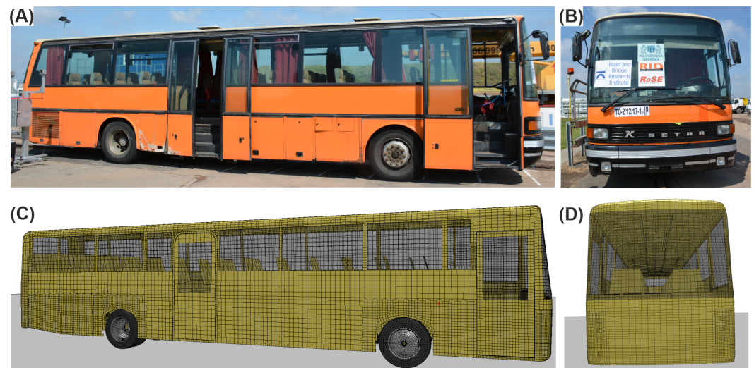
Figure 7. Comparison between the bus used in the experiment and the corresponding numerical model, with (A) a side view of the bus, (B) a front view of the bus, and (C) a side view and (D) a front view of the numerical model.
