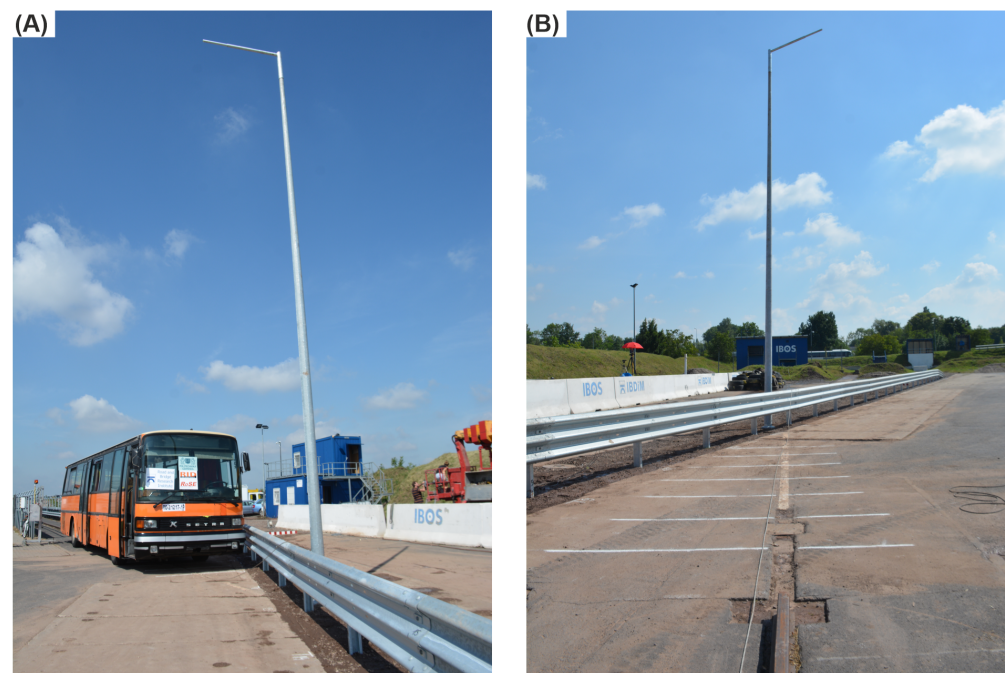
Figure 4. Test site before the collision, with (A) a view of the run-up track with the bus and the impact point and (B) a view of the impact point from the point of view of the run-up track.
