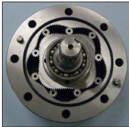
Figure 4. The hydraulic motor with satellite mechanism type 4 \times 5 . The number of teeth: curvature z_E = 130 , rotor z_R = 104 and satellite z_S = 12 , tooth module m = 0,5 \text{ mm} 35,36 .
