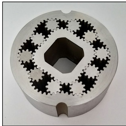
Figure 28. Satellite mechanism type 4 \times 6 : made of metal by WEDM ( z_S = 10 , z_{Rc} = 5.5 , z_R = 44 , z_E = 66 ).
