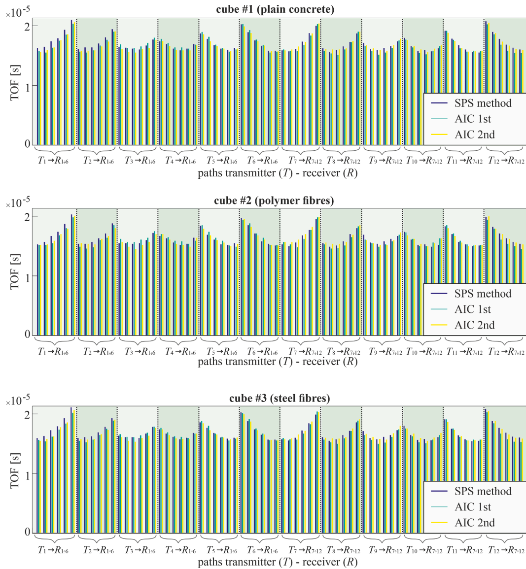
Fig. 8. TOF comparison for signals propagating from transmitters ( T_1 - T_{12} ) to receivers ( R_1 - R_{12} ) determined by SPS, AIC 1st and AIC 2nd methods.
