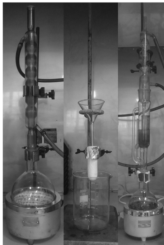
Fig. 2. Experimental glassware setup. From left: precipitation set, filtration set, washing (Soxhlet) set.
