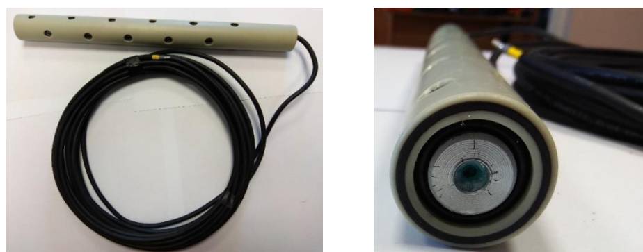
Figure 8. View of a zinc electrode intended for installation within the protection system.
