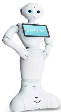
Fig. 2: Pepper, an autonomous semi-humanoid programmable robot, designed with the ability to read emotions. Source: https://www.softbankrobotics.com/emea/en/pepper
