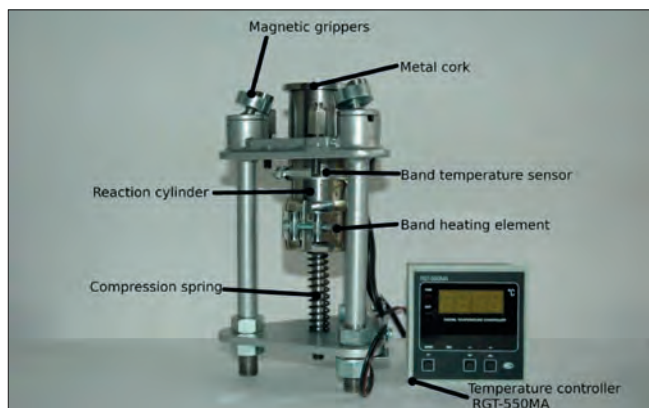
Fig. 6. The KE-2 corrosion tester with some of its elements.
