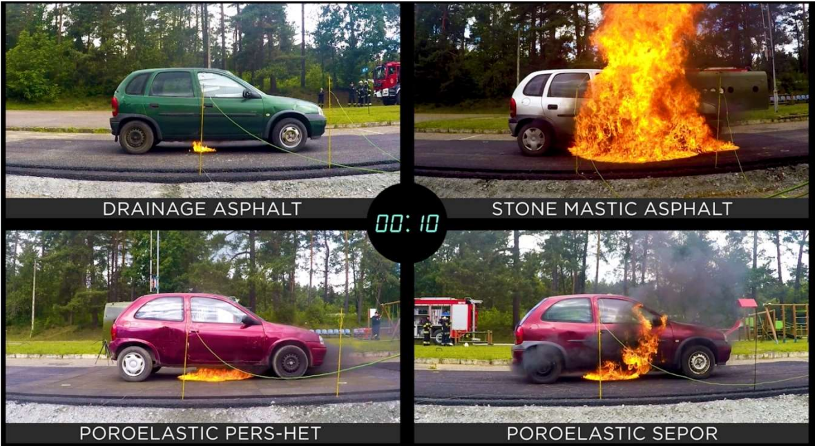
Figure 9. Development of fire 10 s after ignition [27]
