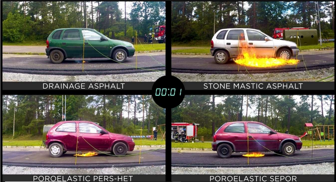
Figure 8. Development of fire 1 s after ignition [27]
