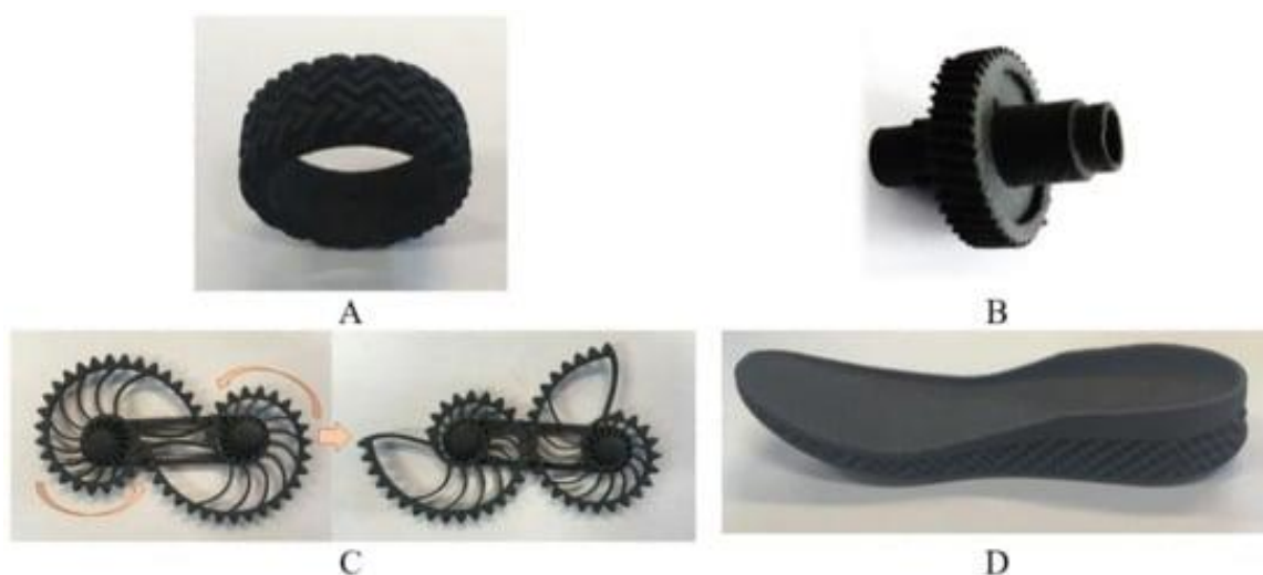
Figure 6. Prototypes 3D printed by selective laser sintering technique: (A–C) tire and complex shape parts based on PA12 with 20 wt.% of ground tire rubber (particle size below 150 \mu\text{m} ) and (D) porous flexible insole based on thermoplastic polyurethane (TPU) with 20 wt.% of ground tire rubber (particle size below 150 \mu\text{m} ) [288].
