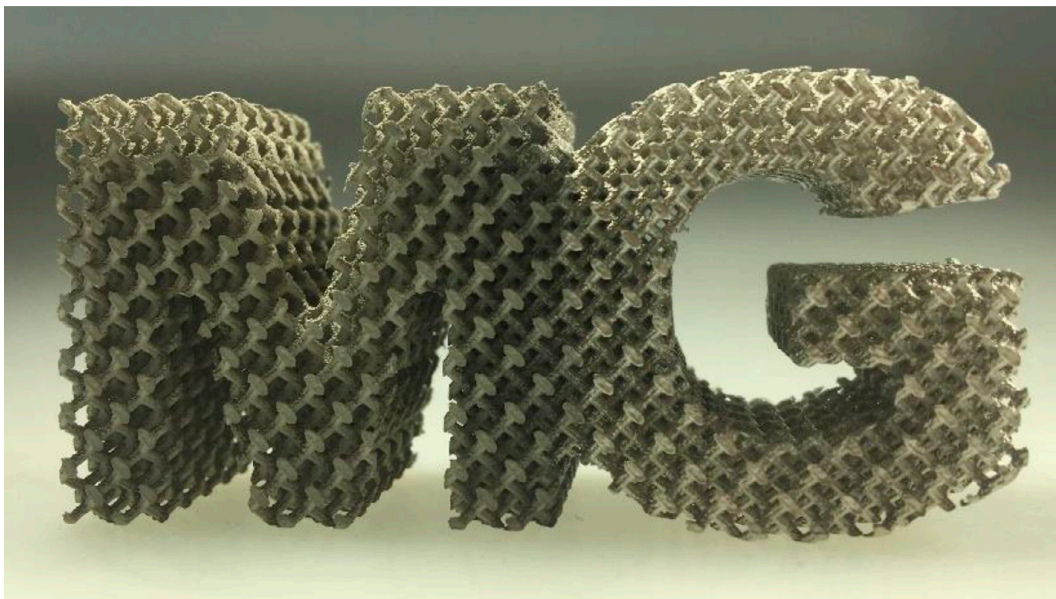
Figure 1. Laser powder-bed fusion (LPBF) created an Mg-shaped lattice structure in a magnesium alloy [27].
