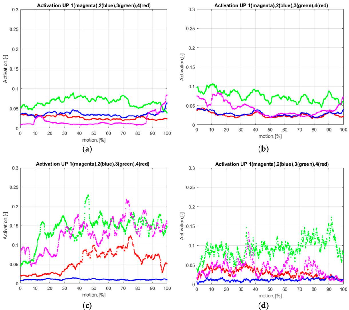
**Figure 4.** EMG data processed (mean value of the RMS normalized data): BB ( $EMG_1$ ), TB ( $EMG_2$ ), AD ( $EMG_3$ ), and UT ( $EMG_4$ ): (a) Reference subject in **motion1** under natural conditions; (b) Reference subject in **motion1** under passive manipulator conditions; (c) DMD subject in **motion1** under natural conditions; (d) DMD subject in **motion1** under passive manipulator conditions.
