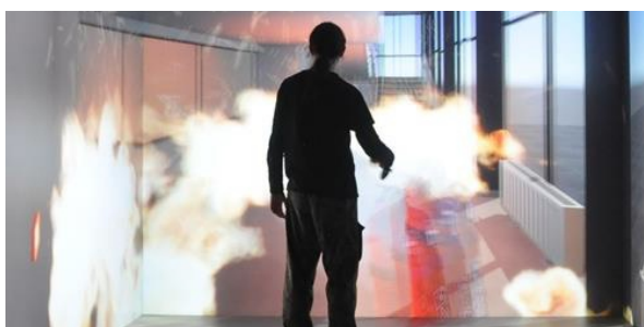
Figure 9: A small fire and extinguisher simulator
