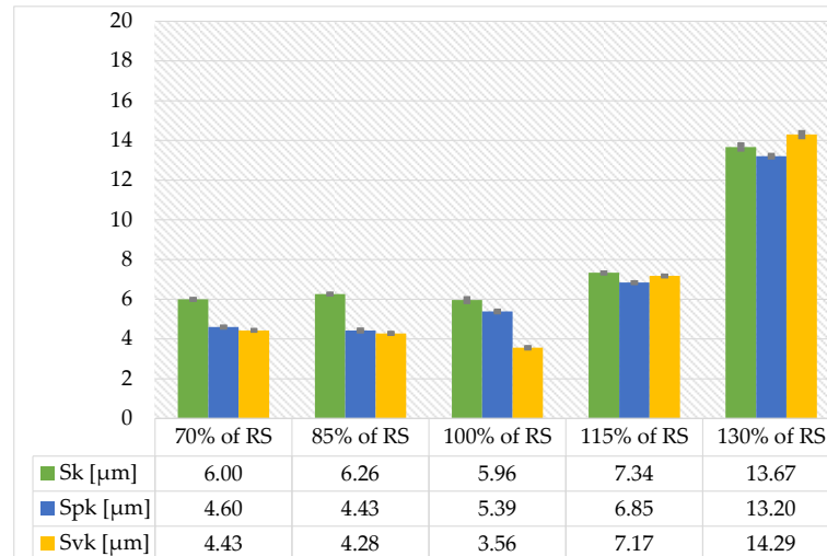
Figure 12. Variation of the Sk, Spk and Svk parameters depending on the cutting speed calculated according to PN-EN ISO 25178-600 [49].
