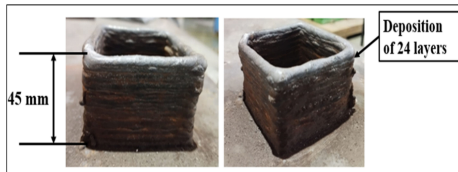
Figure 9. Stainless steel sample deposited with argon shielding gas.
