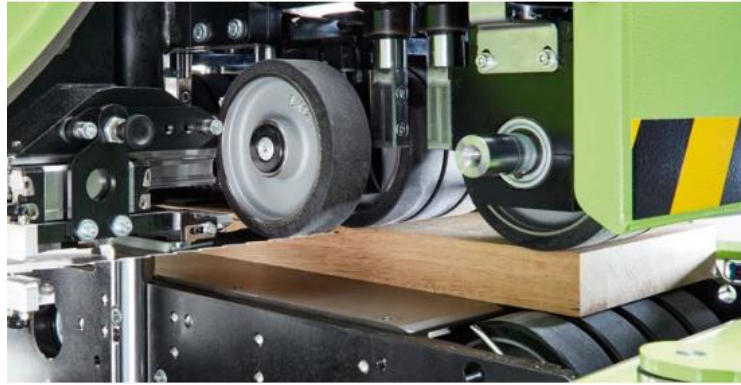
Fig. 3. Cutting zone of the band sawing machine DSB Singlehead NG XM (DSB Singlehead, 2022).
