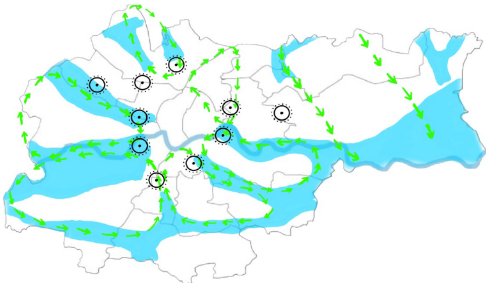
Figure 3. Plan of Cracow with aeration corridors (in blue) and a diagram of the operation of ventilation towers (circulation is marked with arrows), and the potential location of ventilation chimneys (marked with black circles); developed on the basis of [15, 17]
